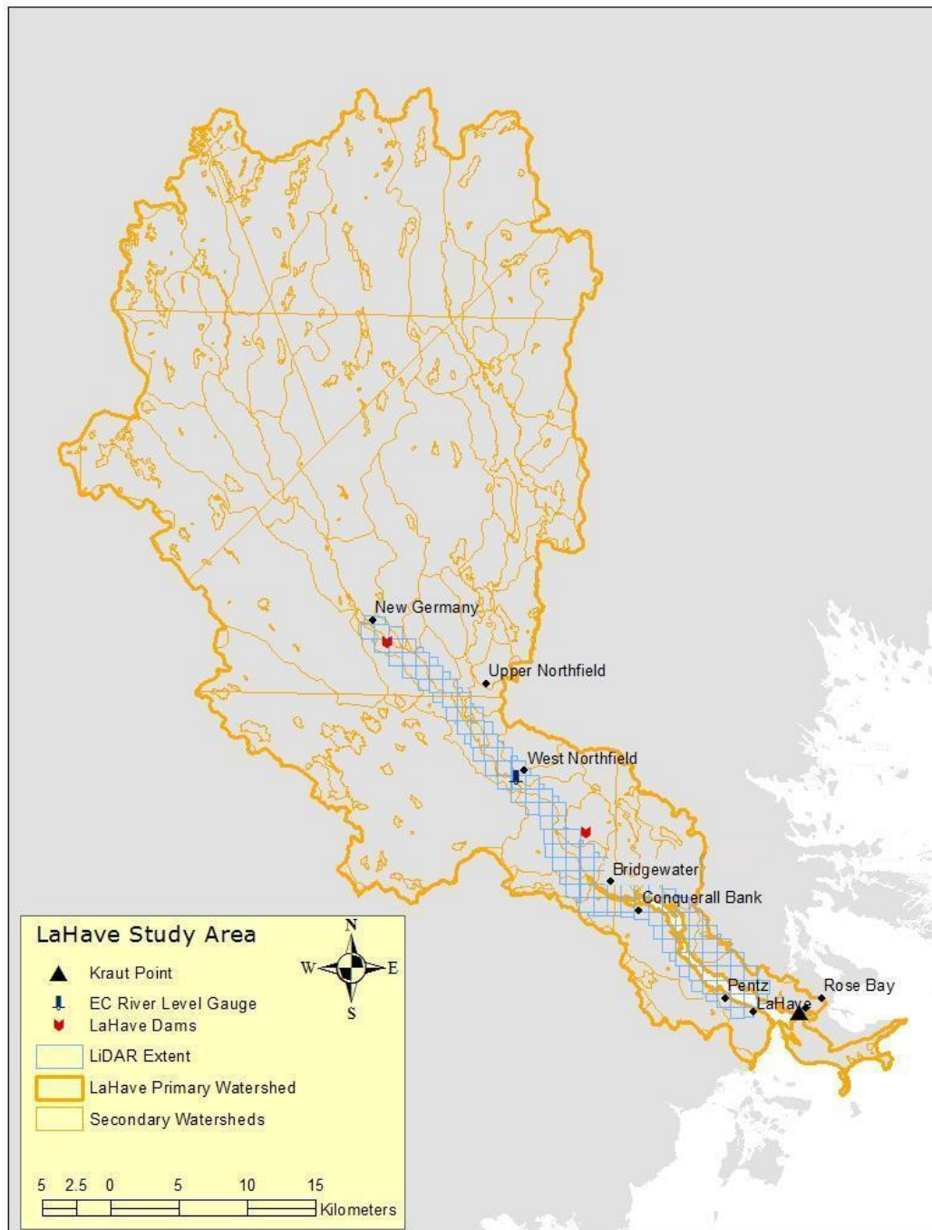
Figure 1:1 LaHave River study area showing the watershed boundary, Kraut Point Harbour (location of AGRG tide gauge), Environment Canada river level gauge at West Northfield, and two dams in the watershed: the Morgan Falls Power Station at New Germany, and a private dam on a LaHave River tributary located north of the Town of Bridgewater.
