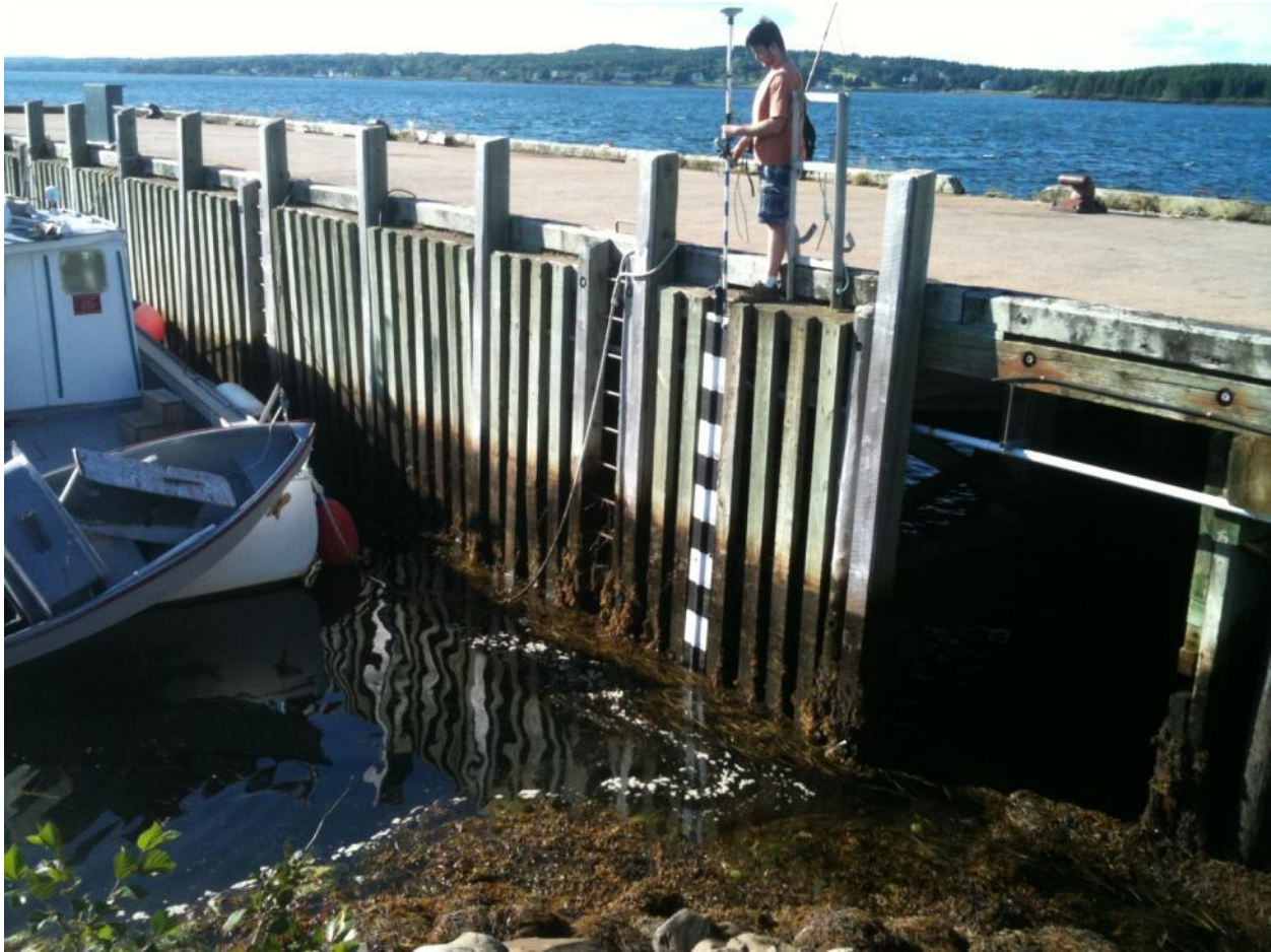
Figure 2:3 Kraut Point tide gauge. Tide board (black and white 10 cm divisions) with the sensor deployed in a PVC tube.
