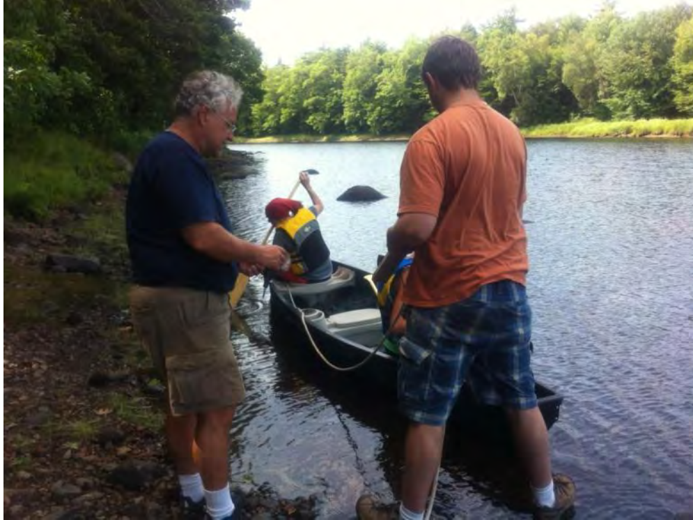
Figure 2:5 AGRG deployed a depth sounder on a canoe to survey the river bed elevations in the LaHave River upstream of Bridgewater.
